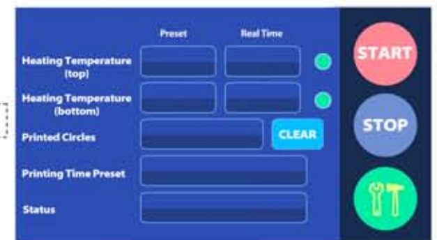
Step 5. Press [start] button to start 3D dye-sublimation process.
