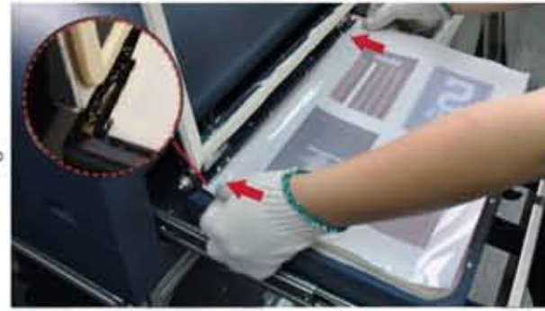
Step 2. Put on the printed film over the cases. Gloss side should be on the top
